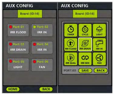
Confirm the device port that requires setting in the port interface at first, and set it as light and other data according to actual needs.
