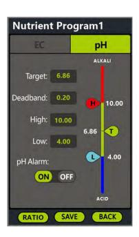
Under the tag of pH, the following information is displayed on the interface: (the maximum set value of pH ranges from 0 to 14.00)
