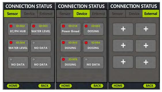
Tags on the interface display relevant information about sensors (Sensor), actuators (Device), and external devices (External) respectively.
