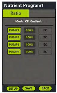
On the interface below the tag of Ratio, if a peristaltic pump expansion device is connected, the corresponding peristaltic pump information will be displayed. By default, only 4 pieces of peristaltic pump information will be displayed on the interface. (up to 8)
