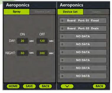
Select the spray mode "Spray" and the port parameter setup "Device Set" on the tags at the top of the interface to switch the setup interface.
