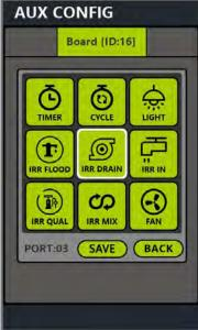
Confirm the device port that requires setting in the port interface at first, and set it as irrigation drain (IRR DRAIN), irrigation backwater, irrigation inflow (IRR in), light, fan and other data according to actual needs.
