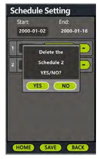
In the periodic table mode, clicking the button "-" on the periodic column can delete the data in the single data column.
