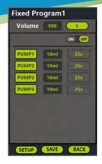
It can set the quantity (Volume) of fertilizer to be added, data unit (L/Gal), receive working test, separate pump effective operation, input data per unit for each pump, expected working time, etc.
