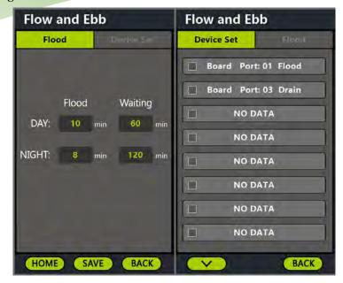
Select the flow mode "Flood" and the ebb mode "Drain" on the tags at the top of the interface to switch the setup interface.
