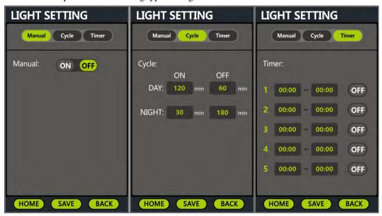
Under the parameter setup of light, there are three different working mode settings: manual mode, cycle mode and timer mode.
