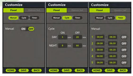
Select the irrigation mode "Flood" on the tag at the top of the interface to set the interface.
